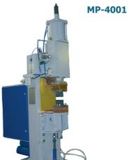
MP-4001 is designed for electrical resistance soldering by copper-phosphorus and silver soldering alloys of copper and copper alloy
