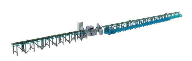
The devices ADFS are designed for automatic arc welding of embedded parts under a layer of flux. Welding of reinforcement steel bars of smooth and periodic profile to flat surfaces of rolled steel is exercised as back-to-back angles. ADFS devices design involves manual load of bars, metal sheets and flux.
